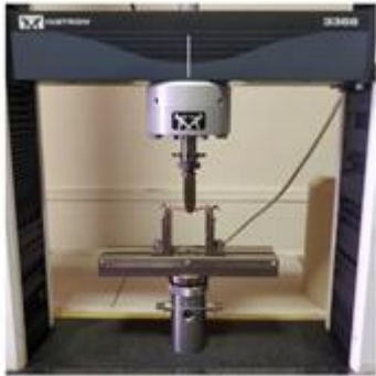
Figure 15: Flexural strength test in Universal testing machine
