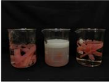
Figure 14: Specimen immersion in distilled water, 8% Rosemary oil and 1% Sodium hypochlorite solutions
