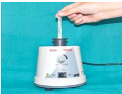
Figure 2: Primer preparation with the help of vortex mixer (10mg of nanoparticle in 1ml of primer).
