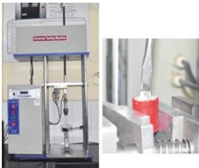
Figure 3: Intron universal testing machine and measurement of shear bond strength.
