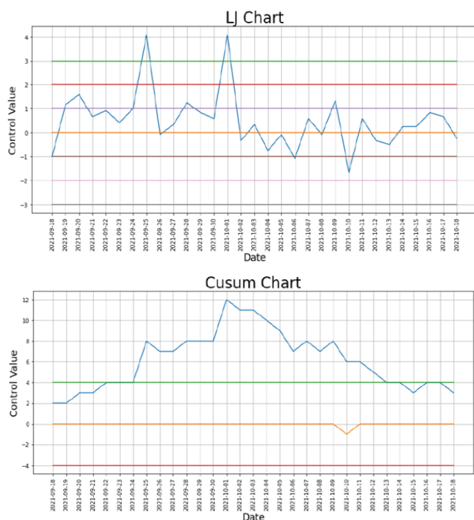
Figure 9: LJ chart of PT showing 13S error on 25/09 and corresponding Cusum chart showing out-of-limit event on 25/09
