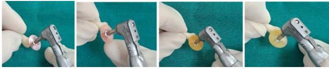
Figure 13: Polishing the samples with Sof-Lex System Discs
