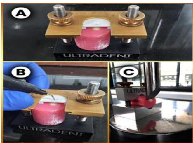
Figure 3: Specimen preparation. (A) An acrylic-resin embedded tooth was mounted onto the bonding clamp and bonding mold. (B) Composite was bonded onto either dentin or enamel surface. (C) Shear bonding test was then performed
